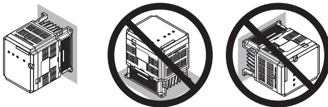
Figure 8 Correct Installation Orientation (Braking Unit)
